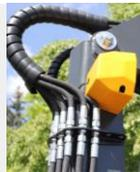
Shut-off valve for lifting cylinder
